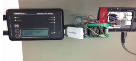
Figure 4: Reading operation under forensic bridge
